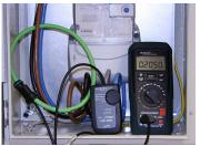
The flexible probe head of ACP 3000 allows quick and easy installation around conductors that may be inaccessible by conventional CTs and clamp meters.
